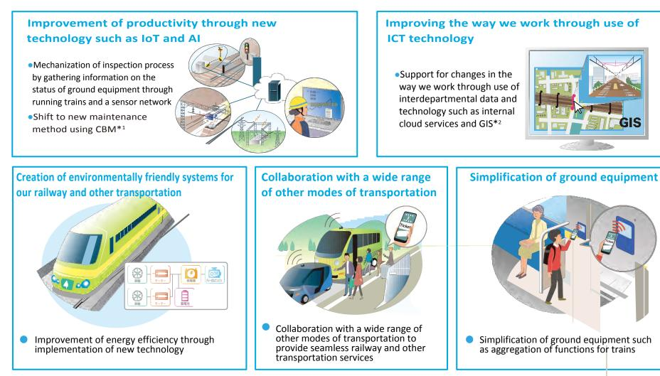
\*1 Condition Based Maintenance: A preventive maintenance principle in which the status of the equipment is ascertained through round-the-clock monitoring so that maintenance is only performed when needed, balancing quality with efficiency \*2 GIS: Geographic Information System
