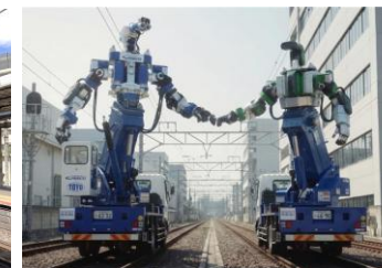
Multi-purpose railway heavy machinery ZIZAI
