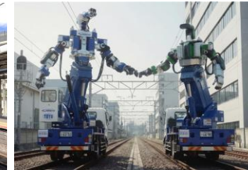
Multi-purpose railway heavy machinery ZIZAI
