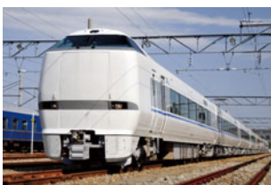
Thunderbird limited express Operating section : Osaka – Kanazawa, Wakura-onsen Typical train configuration : 9 cars Maximum speed : 130km/h
