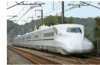
Sanyo and Kyushu Shinkansen N700 Operating section : Shin-Osaka – Kagoshima-Chuo Train configuration : 8 cars Maximum speed : 300km/h
