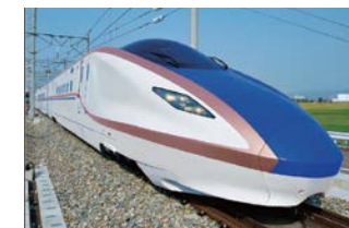
Hokuriku Shinkansen W7 Operating section : Tokyo – Kanazawa Train configuration : 12 cars Maximum speed : 260km/h
