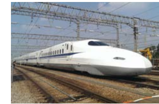
Tokaido and Sanyo Shinkansen N700A Operating section : Tokyo – Hakata Train configuration : 16 cars Maximum speed : 300km/h
