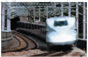
Nozomi N700 Typical train configuration 16 cars Capacity 1,323 Maximum speed 300km/h
