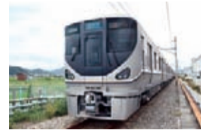
225 series commuter train Typical train configuration 8 cars Capacity 1,091 Maximum speed 130km/h
