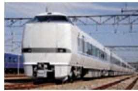
Thunderbird limited express Typical train configuration 9 cars Capacity 546 Maximum speed 130km/h
