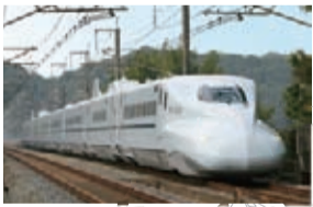
Sakura/Mizuho N700 Typical train configuration 8 cars Capacity 546 Maximum speed 300km/h
