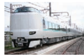
Kuroshio limited express Typical train configuration 6 cars Capacity 360 Maximum speed 130km/h
