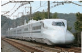
Sakura/Mizuho N700 Typical train configuration 8 cars Capacity 546 Maximum speed 300km/h
