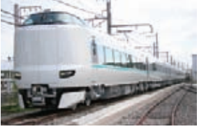
Kuroshio limited express Typical train configuration 6 cars Capacity 360 Maximum speed 130km/h
