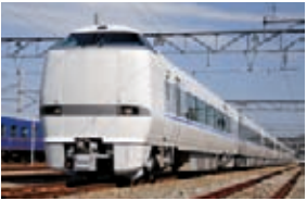
Thunderbird limited express Typical train configuration 9 cars Capacity 546 Maximum speed 130km/h
