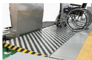
Wheelchair step elimination mechanism for eliminating the level difference when getting on and off the railcar
