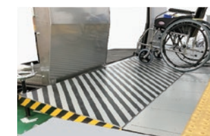
Wheelchair step elimination mechanism for eliminating the level difference when getting on and off the railcar
