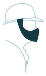
FREE MOUTH SHIELD FOR CONSTRUCTION WORKER is the mouth shield for construction workers. For heat stroke prevention and stress-free, this shield is deigned to be keep away from the face. Anyone can easily make this shield from a commercially available A4 size clear file folder.
