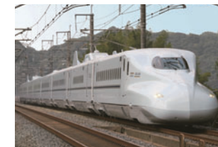
Sanyo and Kyushu Shinkansen N700 Operating section : Shin-Osaka – Kagoshima-Chuo Train configuration : 8 cars Maximum speed : 300km/h
