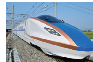
Hokuriku Shinkansen W7 Operating section : Tokyo – Kanazawa Train configuration : 12 cars Maximum speed : 260km/h
