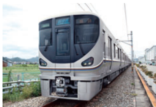
225 series commuter train Operating section : Kansai Urban Area Typical train configuration : 8 cars Maximum speed : 130km/h
