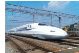
Tokaido and Sanyo Shinkansen N700A Operating section : Tokyo – Hakata Train configuration : 16 cars Maximum speed : 300km/h
