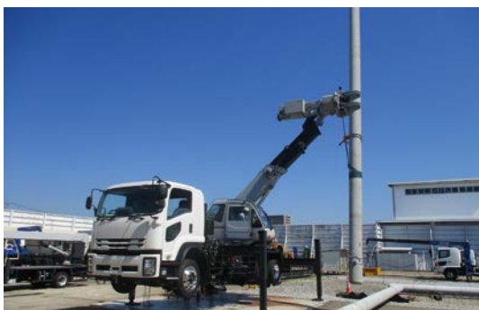
Utility pole handling vehicles
