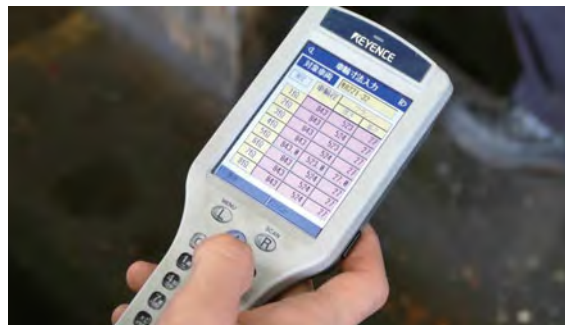
Handy terminal (Display of required inspection items and instant analysis of input results)
