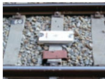
JR-West is installing ATS equipment for preventing accidents due to excessive speed.
